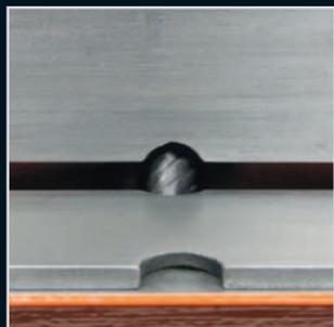
Position I: Material thickness from 4.5 mm
