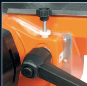
Fine adjustments to milling depth/
