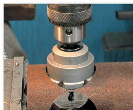
Drilling in pipes
