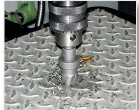
Drilling structured sheet metals
