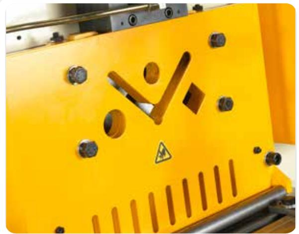
Angle shearing without loss of material.
