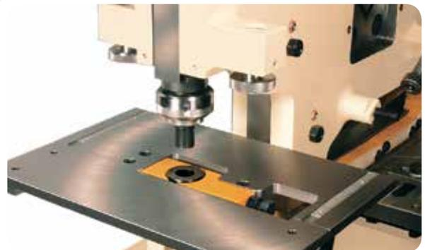
Goose neck die-holder for punching of L and I sections on legs and webs. Quick tool change.
